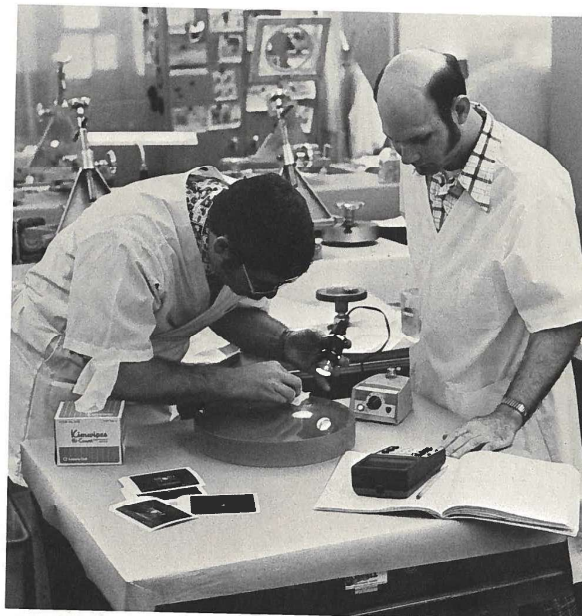
The heliostat mirror being prepared in the optical shops of the University of Arizona.
