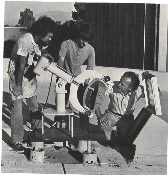
18 Dr. Stephen Jacobs of the Optical Sciences Center and Planetarium technicians align the heliostat mirror.
